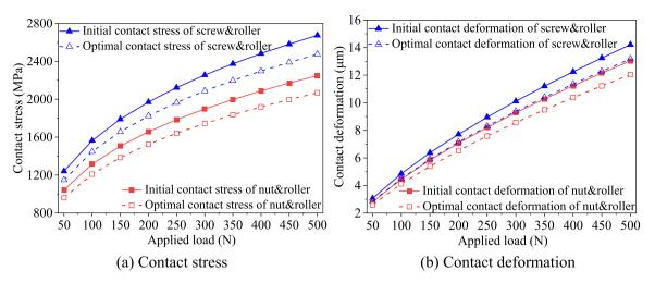
Fig. 13. Contact stress and deformation on helical surfaces after structural design.
