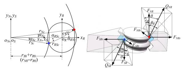
Fig. 2. Static force analysis at contact points.
