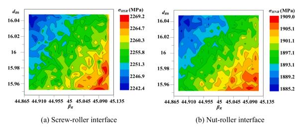
**Fig. 10.** Contour map of contact stress affected by  $d_{R0}$  and  $\beta_{R}$ .
