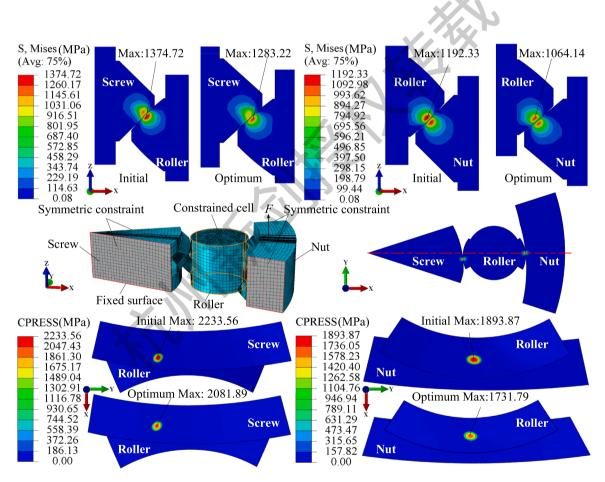
Fig. 14. Comparison of the contact characteristics between the initial and optimized PRSM by FEM.
