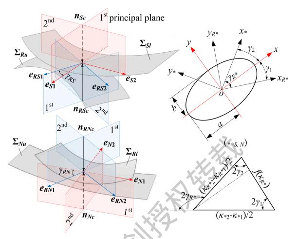
Fig. 3. Local contact geometry.
