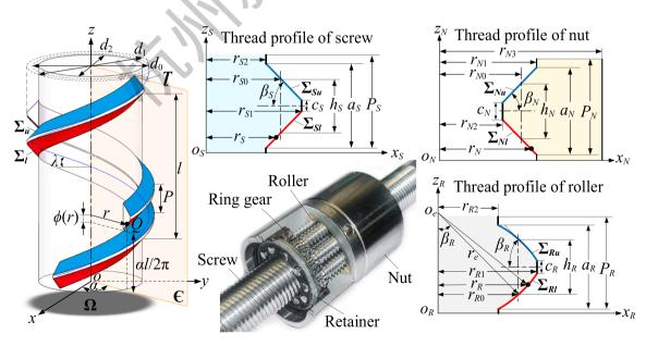
Fig. 1. Structural diagram and independent part coordinate systems of PRSM.
